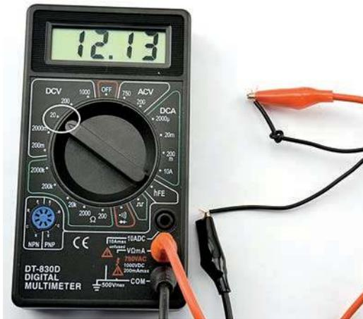
**FIGURE 1-13** Using a multimeter to find the power supply polarity
