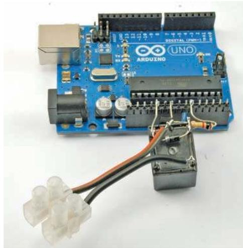
**FIGURE 6-9** The Arduino relay interface
