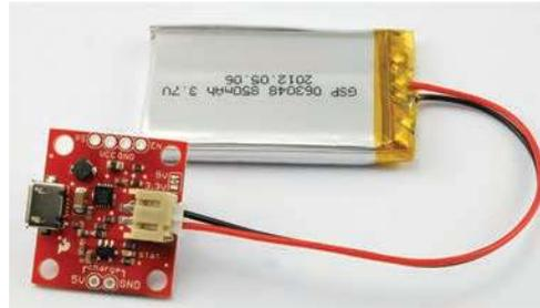
**FIGURE 5-10** Combined LiPo charger and booster
