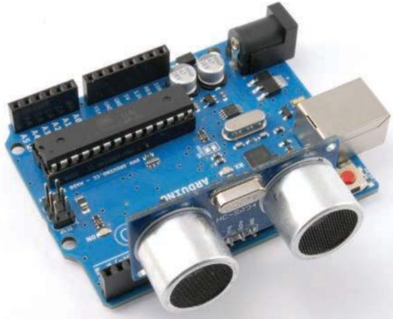
**FIGURE 8-10** An HC-SR04 rangefinder on an Arduino
