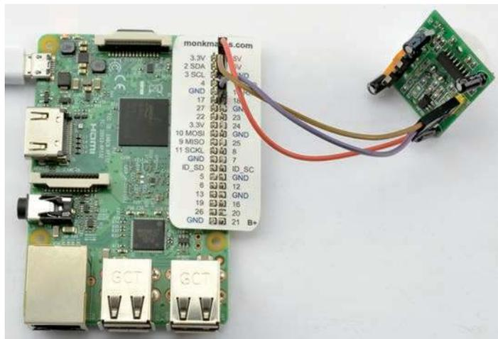
To use with a Raspberry Pi, you will need female-to-female jumper wires connected as follows:
