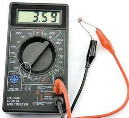
**FIGURE 3-8** Measuring the LDR resistance
