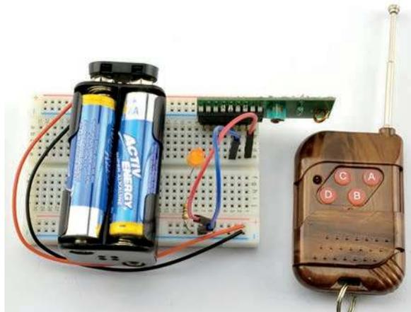
**FIGURE 8-12** An RF module on breadboard
