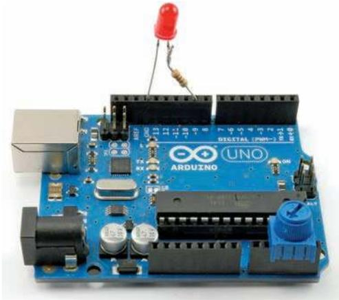
**FIGURE 6-20** An Arduino, variable resistor, and LED
