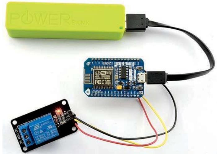
that the NodeMCU board is powered by USB cable to a 5V backup battery.
