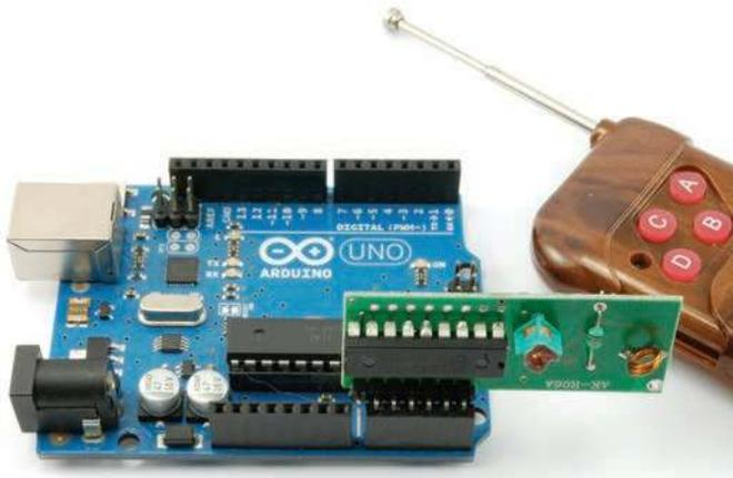
**FIGURE 8-14** Using a RF remote with an Arduino
