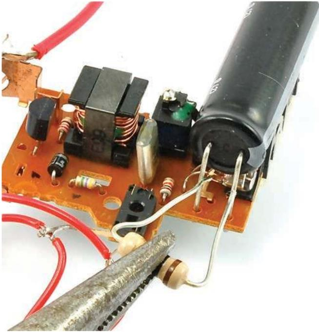
**FIGURE 11-1** Safely discharging a capacitor
