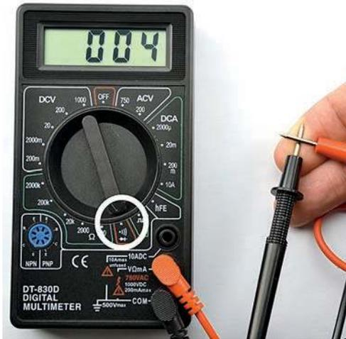
**FIGURE 1-8** A multimeter in Continuity mode
