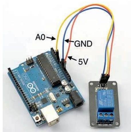
FIGURE 6-12 Connecting a ready-made relay module to an Arduino
