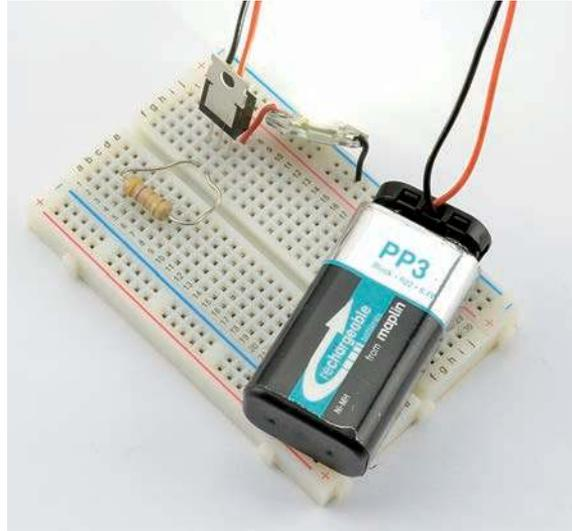
You will need to solder lengths of solid-core wire to the LED's terminals so it can plug into the breadboard. It is a good idea to leave the insulation on so there is no chance of the bare wires touching the heat sink and shorting. Using different colors of wire insulation also allows you to tell which lead is positive.
