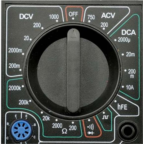
**FIGURE 12-1** Multimeter range selection
