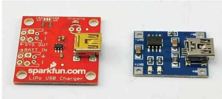
components. However, there are plenty of ready-made modules available, many of which use the MCP73831 IC. Figure 5-4 shows two of these—one from SparkFun (see the Appendix, M16) and one for just a few dollars from eBay.
