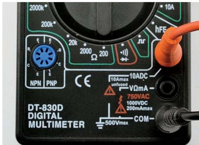
voltage sockets, as these are more likely to be used next. If you try and measure current with the leads in the voltage sockets, then all that will happen is that you get a reading of zero.
