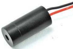
**FIGURE 4-30** A laser diode module
