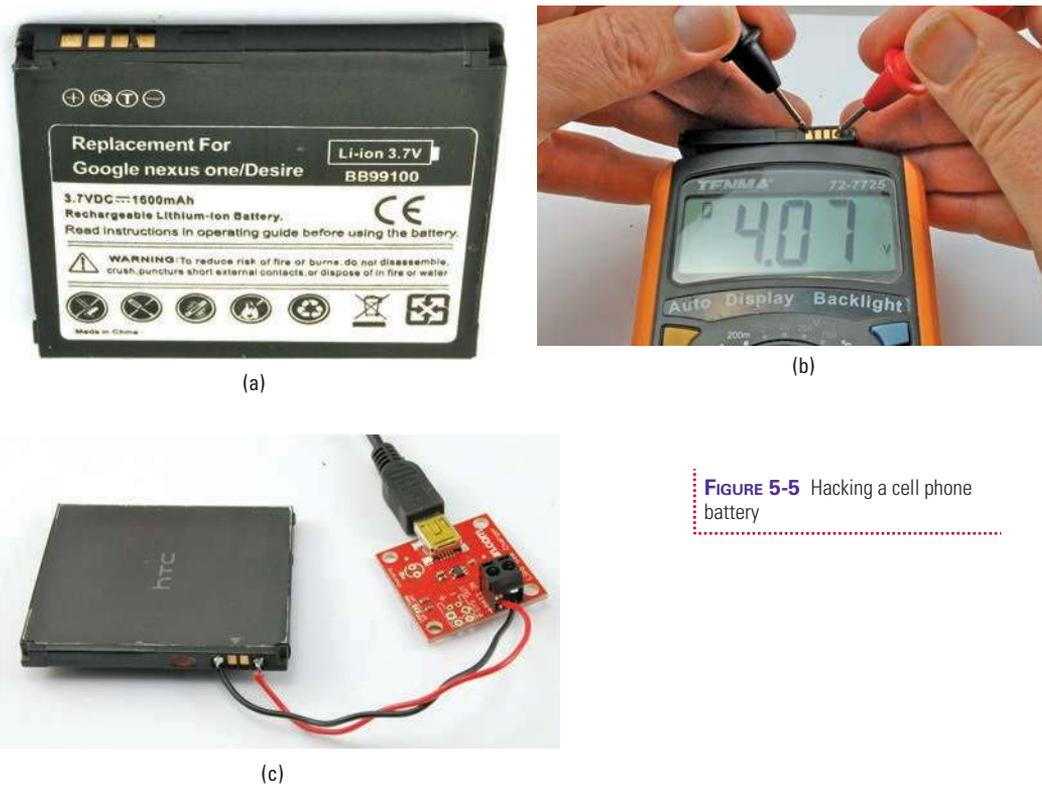
FIGURE 5-5 Hacking a cell phone battery
